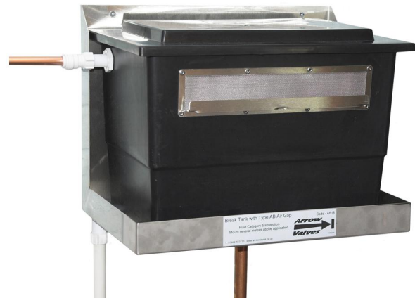
AB18T – Rainwater header with Type AB air gap. Supplied complete with stainless steel screened slot, wall bracket incorporating drip tray. Also supplied – two float valves and two servicing valves
