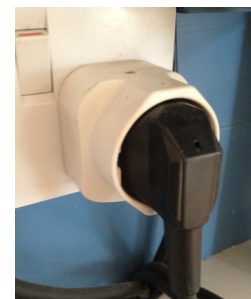
Solenoid cable plugged directly into adaptor
