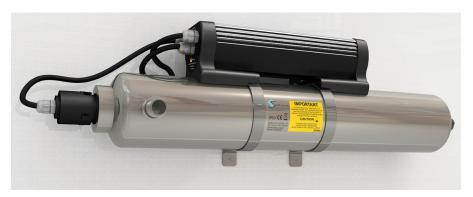
The UV disinfection unit is designed to sterilise harvested rainwater and is required is certain situations where there is deemed to be a risk to users from water-borne organisms. It works by breaking down the organisms' DNA as a result of exposure to a particular part of the spectrum of light radiation.
