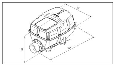
Electronic device for the electric pumps control based on inverter technology. It controls the starting and stopping of the electric pump and modulates the motor rotations according to the water request from the system.
