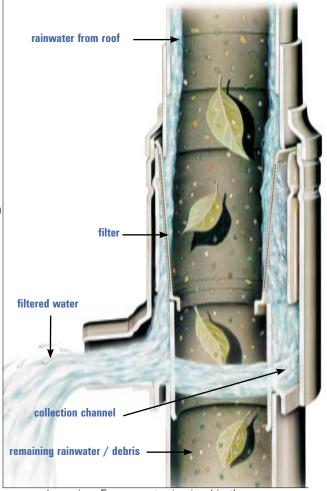
downpipe. Excess water is piped in the conventional manner to surface water drain or soakaway.
