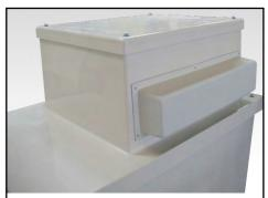
Raised valve housing with screened weir overflow giving a type AB air gap, can be fitted with drop-arm equilibrium float valve or Keraflo valve.
