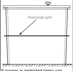
If access is restricted tanks can be supplied in two parts with a horizontal split, enabling movement into or through tight spaces.
