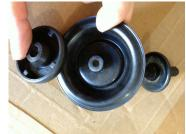
Replace the diaphragm assembly into the unit and then fit the spring and housing cap onto the main body.
